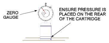
Figure 3-18. Zeroing the Micrometer Gauge.
